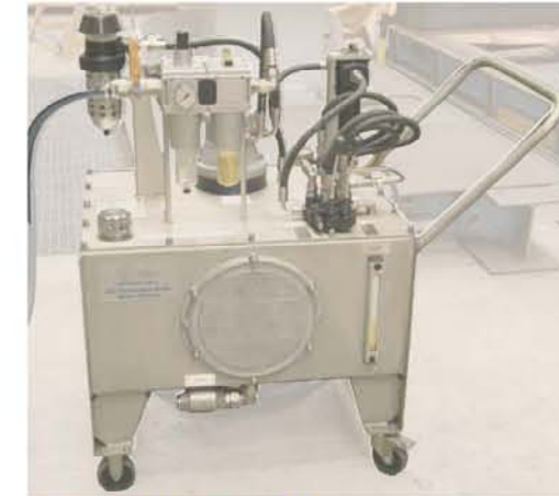
Hydraulic Backup System
