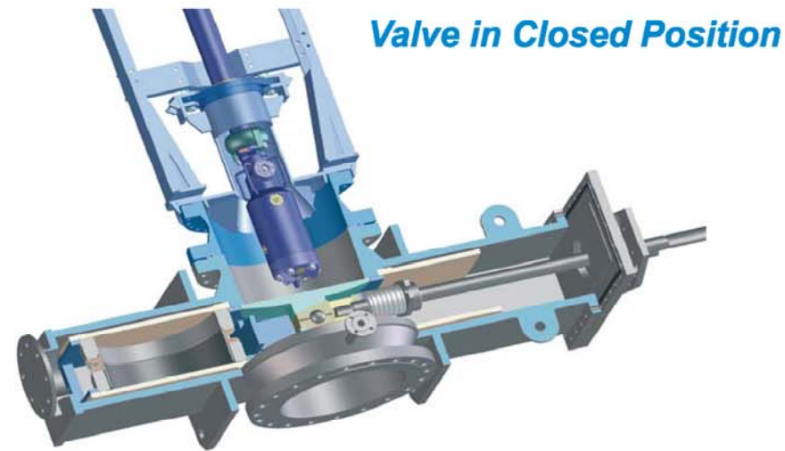
Top Unheading Valve Installation with Cutting Equipment
